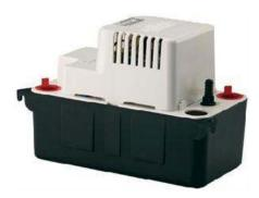
Condensate is produced at a rate of up to a gallon per hour by a residential central air conditioning unit or gas condensing furnace. The installer will feed the condensate from the appliance drain into one of the pumps inlet ports. Condensate pumps are typically equipped to connect with 3/8" ID plastic tubing. The tubing is connected to the pump check valve, leading to a drain line, sump, French drain or laundry sink.
